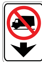
Signs that show a lane in which heavy trucks must not travel
