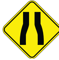
Pavement narrows ahead
