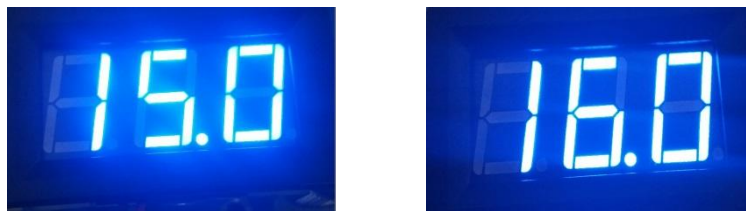
Figure 5-15 Ultra-capacitor's voltage before and after charging.
