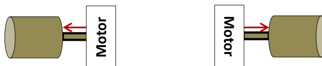
Figure 4-9 Two in-wheel hub motors driving the wheels through very small drive shafts.
