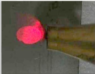
Beam Out of Alignment
